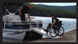
SELF DEPLOYING PONTOON BOAT RAMP
